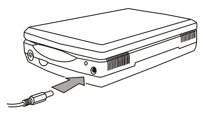
Plugging the power adapter into the SAPPHIRE
