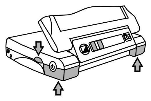
Place index finger in small recessed area and push up with thumb to open the writing stand
