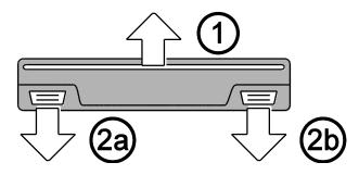
2. The unit is spring loaded and opens to its full reading position. If the unit is off, it automatically turns on when the reading stand opens.
